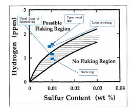
Although the chart above (R. J. Fruehan, *Iron & Steelmaker*, 1997)—adapted to the specificities of the Tihange 2 RPV—is mainly indicative, both the upper and lower shells of the Tihange 2 RPV shell are in the possible flaking region.
