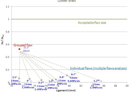
The results of such 3D calculations for the 7 ungrouped flaws show a significant increase of the margin with respect to the maximum allowable size. Similar conclusion is also valid for Tihange 2 grouped flaws.
