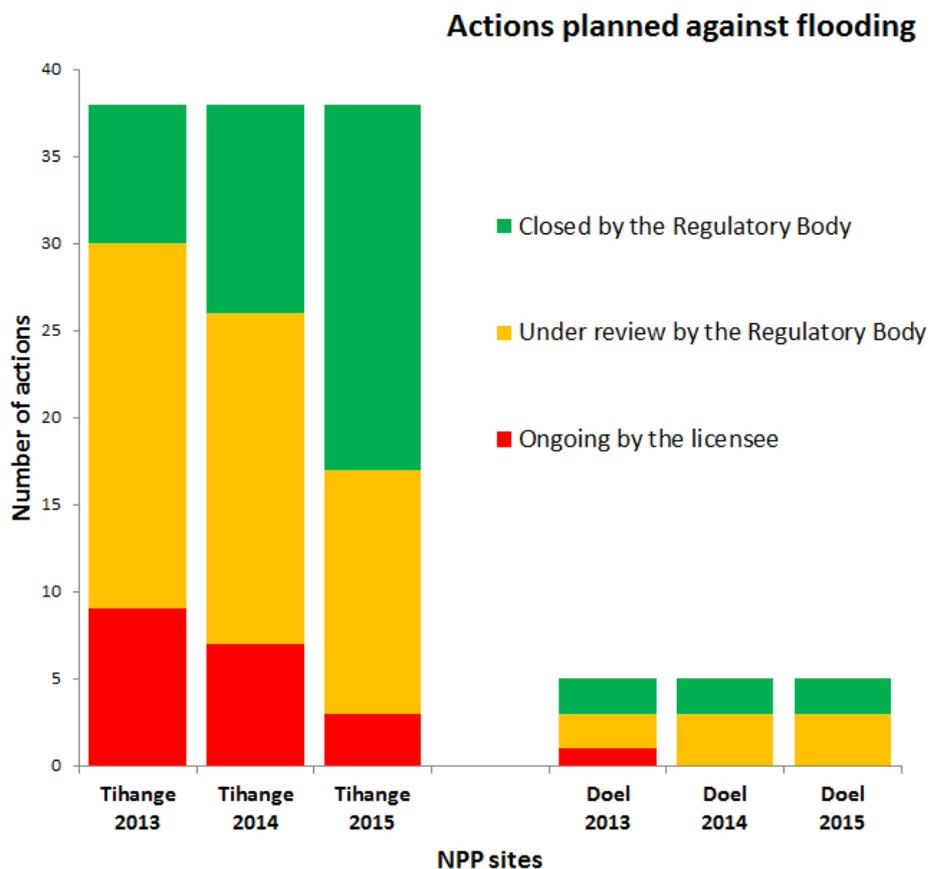
Figure 3 : Evolution of the resolution of the actions concerning the protection against flooding between 2013 and 2015.
